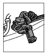
In very cold weather, 0°F (-18°C) or colder, the engine coolant heater can help. You'll get easier starting and better fuel economy during engine warm-up.
